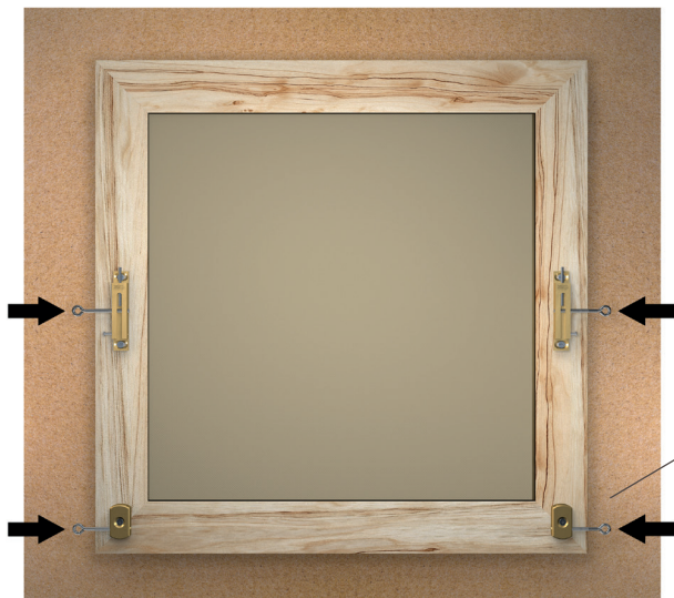
The ring screw shows where the wholes have to be drilled in the pannel on which the artwork is placed.
